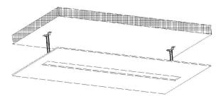
Put the product through the slotted hole of the holiday flower and insert the screw into the fixing plate hole of the product, and then lock it with the screw. (it is recommended that two people operate at the same time)
