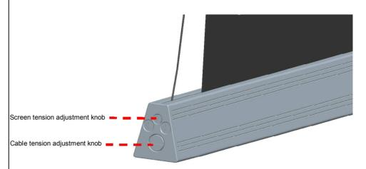
When the black surface under the curtain surface for a long time is uneven, such as corrugations, the screwdriver can turn the screw clockwise to solve this problem.
